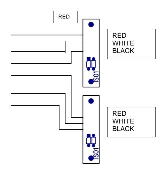
Example showing how to connect PRS600 to AUX Input connector CN5 on PRN607-S standard board.
